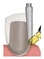
For best results with Procera® restoration, the prep design should allow access for the scanning probe. (See image on the left)
