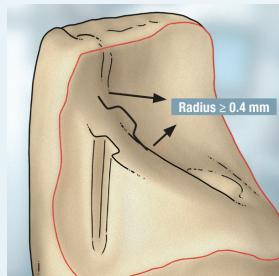
Figure 2: Retentive element: rounded ridge (Radius  $\geq 0.4$  mm).
